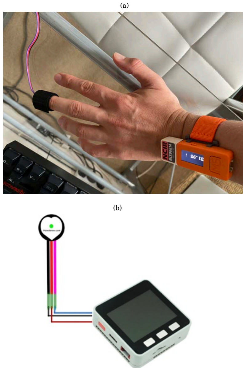
FIGURE 8.4. (a) Participants wearing NCIR sensor on wrist to gauge temperature and PulseSensor finger strap on a pulse point to take all heart rate data. (b) The PulseSensor circuit diagram - with ground in black wire, 5V power red wire and pink-blue data wire.
